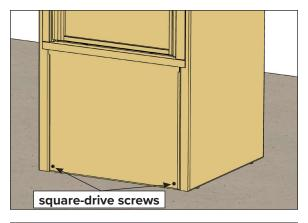
2). Pull the panel out at the bottom and down from behind the PORT package-box trim.
